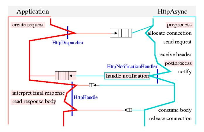
Preprocessing and postprocessing are done by background threads, as is consuming the response. Postprocessing is done before notification, since that is the last chance to detect and report a problem in a background thread.
