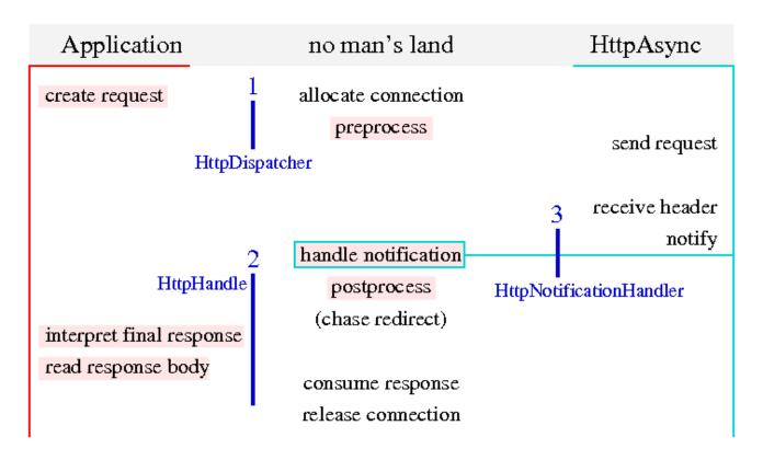
Two of the interfaces are application-facing. HttpDispatcher is used to transfer control over a request to HttpDispatch. Since this is done by a call from an application thread, the implementation can then execute code in that application thread. Eventually, the request has to be passed to the background threads that handle the asynchronous communication. The application obtains an instance of the second interface as a result of the call to HttpDispatch er.
