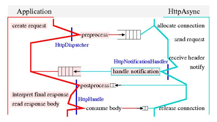
Preprocessing and postprocessing is done by application threads because these steps execute application code. Consuming the response is also done by an application thread, because it is a potentially long-running task that does not necessarily have to be executed by a background thread.
