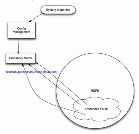
Currently only configuration for injected faults is available. Configuration management allows you to set expectations for faults to happen. The settings can be applied either statically (in advance) or in runtime. The desired level of faults in the framework can be configured two ways:
