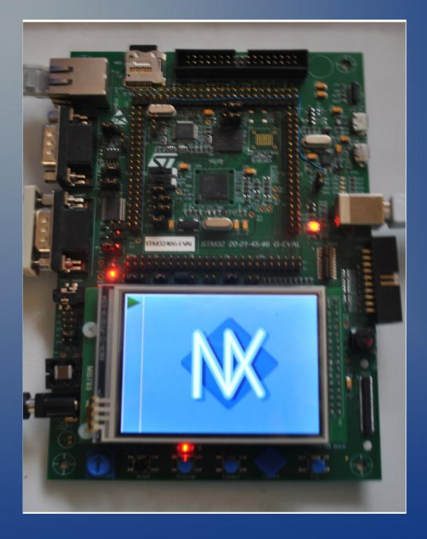
These slides provide screen shots showing the NxWM Unit Test code running on an STMicro STM3240G-EVAL board (as shown)
