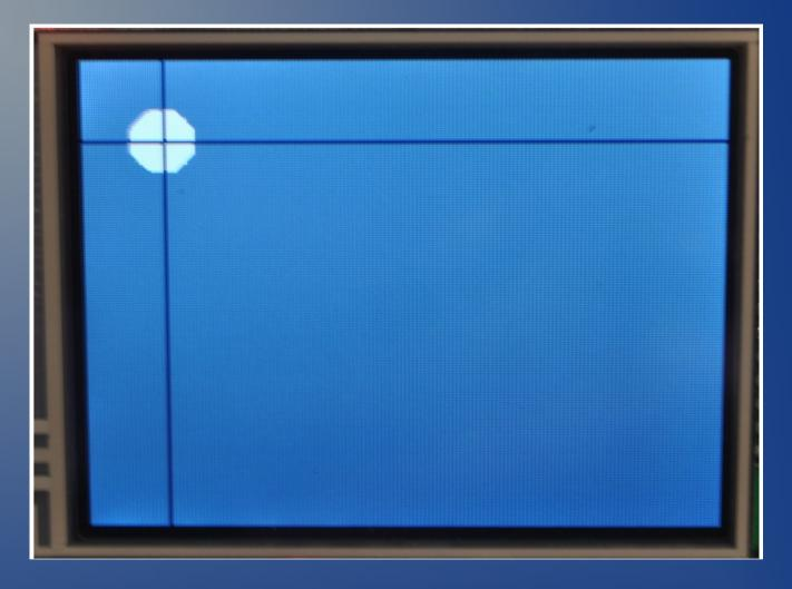
When the test program first comes up, it will expect you to perform a touchscreen calibration. It will present the circle in the cross-hairs at four different positions. You simply have to touch each position. Then the touchscreen is calibrated and you will be presented with the opening screen.
