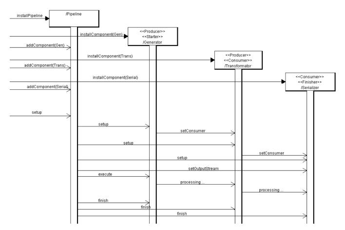
The third block is the heart and soul of cocoon. All the prerequisites have been fulfilled and the pipeline has been set up. It can now start its work and does so by calling a setup method of its components (which have been added by the Invocation). During the setup phase, a component can do specific things that have to be set up before the pipeline is executed, these are certain parameters, which can be set before, and the method setConsumer, which 'sticks' the pipeline-components together.
