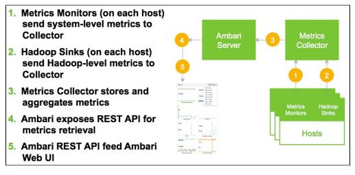
The **Metrics Collector** is daemon that receives data from registered publishers (the **Monitors** and **Sinks**). The Collector itself is build using Hadoop technologies such as HBase Phoenix and ATS. The Collector can store data on the local filesystem (referred to as "embedded mode") or use an external HDFS (referred to as "distributed mode").
