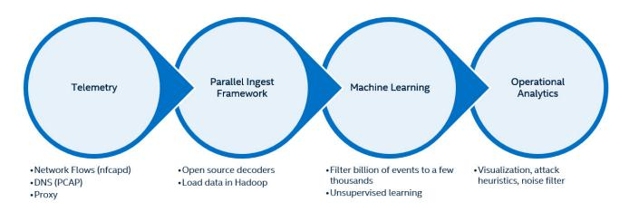
**Parallel Ingest Framework**. The system uses decoders optimized from open source, that decodes binary flow and packet data, then loading the data in HDFS and data structures inside Hadoop. The decoded data is stored in multiple formats so it is available for searching, used by machine learning, transfer to law enforcement, or inputs to other systems.
